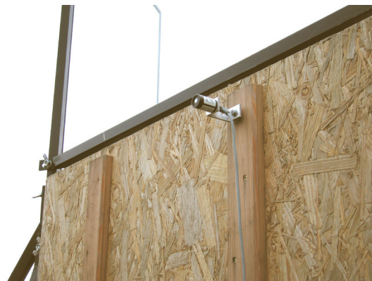
Figure 9: Pyranometer 2 for measuring radiation behind the experimental panes
