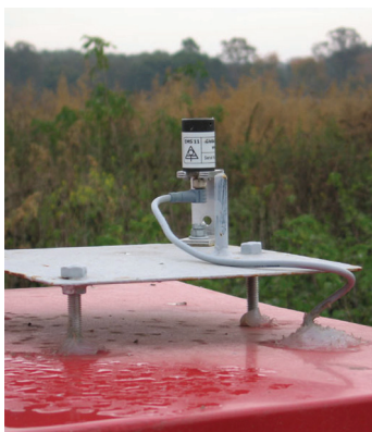
Figure 8: Pyranometer 1 for measuring global radiation
