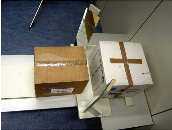
Figure 2: In the lab, the suitability of mirrors was tested in simplified experiments, and a favourable optical path was determined.
