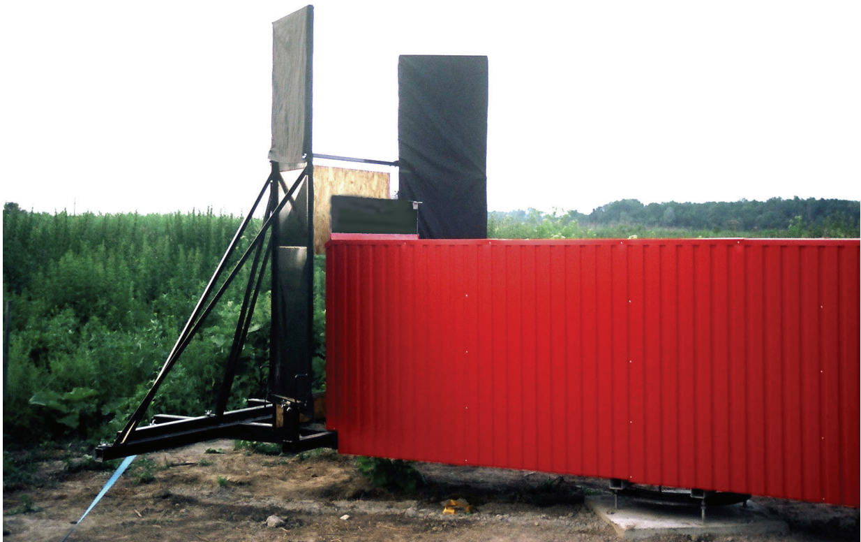
Figure 1: A new experimental tunnel (Flight Tunnel II) in Hohenau-Ringelsdorf serves to continue the research of the years 2004 and 2005 with enhanced facilities, in order to enable better prognoses of the efficiency of markings to reduce bird strikes against glass planes. Flight tunnel II, here not in use, mirrors covered.
