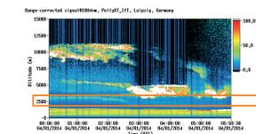
Lidar PollyXT Leipzig time series of range corrected signal aerosol layer: 2.5 - 3.5 km
