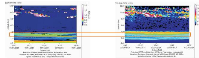
Lidar RALI Bucharest time series of range corrected signal aerosol layer: 2.5 - 4.0 km
