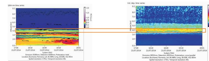
Lidar RALI Bucharest time series of volume depolarisation ratio aerosol layer: 3.5 - 4.5 km
